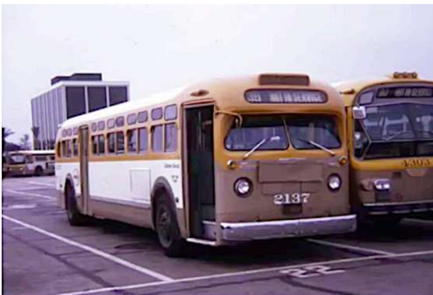
A GM and a new look Flxible. Both had air-ride suspension and GM-made engines. The older GM-style bus on your left was built for 29 years and were dependable and tough. This is a picture from the transition era in Los Angeles. Flxible buses, unlike their GM counterpart brother buses, did have 3 lights in front of their vehicles.
