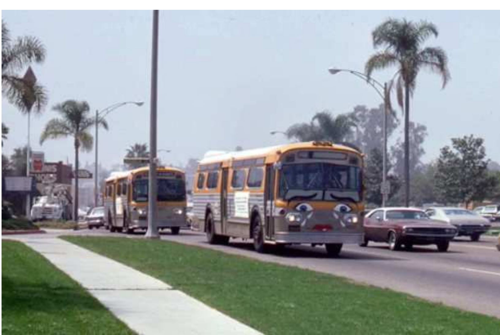
A set of Flxible buses. They were built in either Ohio or Alabama. End of an era. Production ended in 1978 yet, were seen as late as 1992. These are Ohio built buses; Alabama buses had only 2 headlights. Good bye Flxibles.
